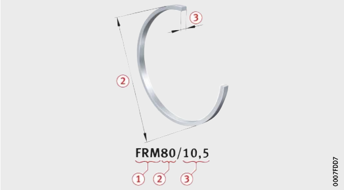
Figure 9 Designation structure of locating rings, example
